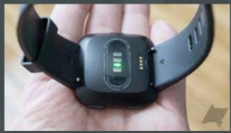
Figure 1: The back of a Fitbit Versa illustrating red, green, and infrared LEDs and detectors.
